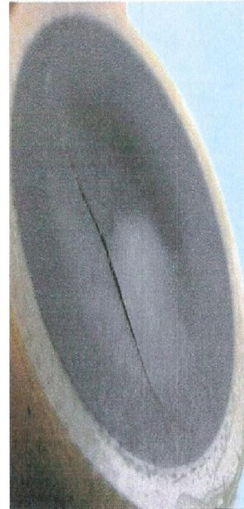
FIGURE 1. Cracked transducer front face due to an excessive applied power (about twice the maximal acceptable excitation level)
