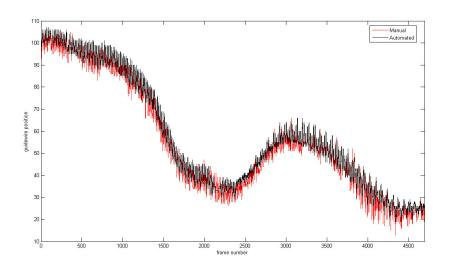
Match between ConDensation tracking estimate and manual marked guidewire position.
