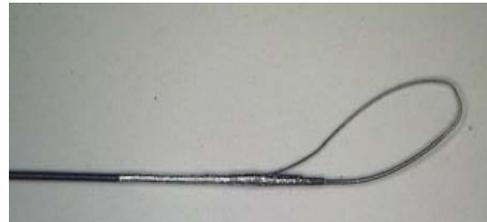
Nitinol Ribbon (0.0014- x 0.006-in.) to Nitinol Tube (0.008-in. OD)
