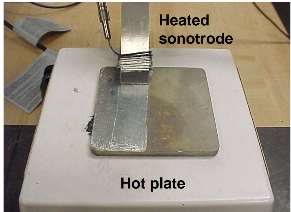
Ultrasonic pretinning oxidized Ti-6Al-4V
