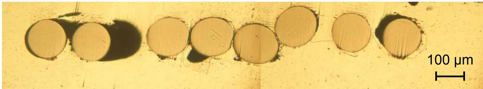
**Material Section of 22.3% NiTi-Al Composite**
