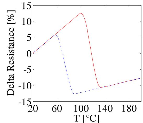
**0 N Load and 12N Load NiTi Wire Model**
