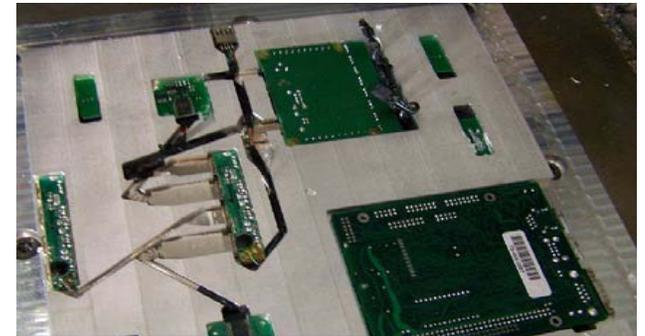
**Electronics Positioned for Embedding\***
