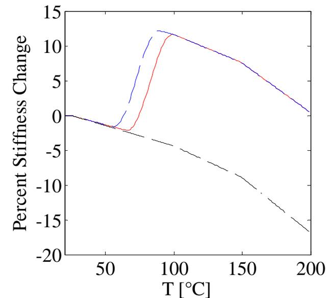
Modeled Stiffness Change of 4.5% , 13.4%, and 22.3% NiTi Area Ratio Composites
