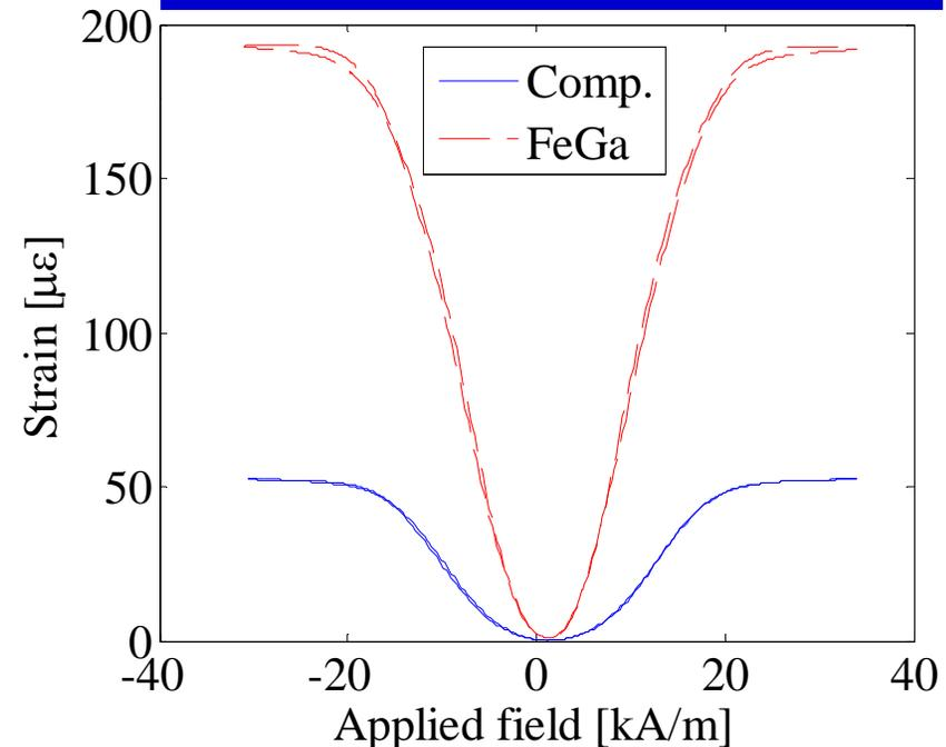
FeGa and FeGa-Al Composite Strain Response to Applied Field
