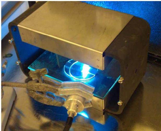
Fragile PMN-PT materials need **low temperature and pressure** for bonding electrical interconnects
