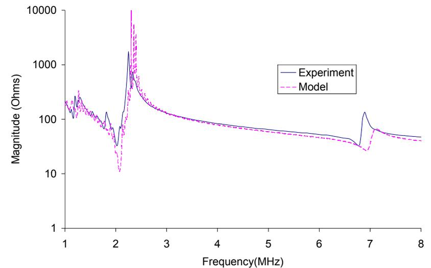
PMN-PT Model was more challenging to match to the experiment matches with experimental test
