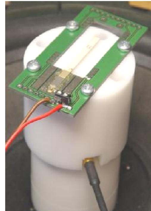
Energy harvesting device mounted on the shaker
