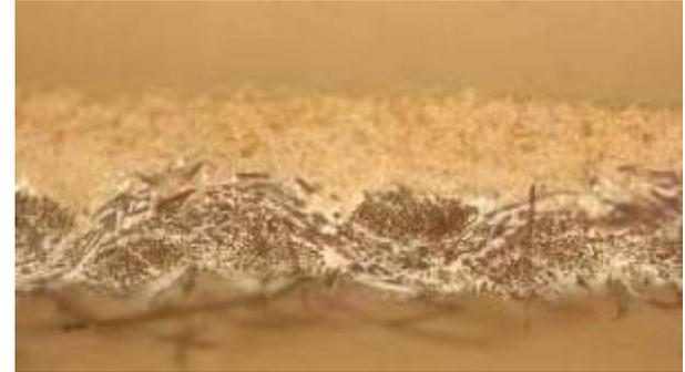
Cross section: Thick film on fabric
