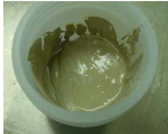
Fabricated piezoelectric paste
