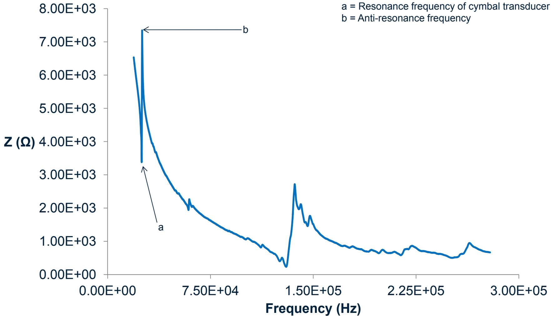
Impedance-Frequency Spectrum of the Modified Brass Cymbal Transducer
