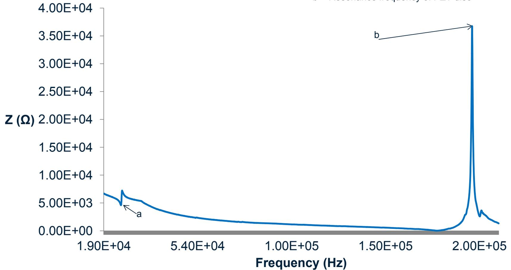
Impedance-Frequency Spectrum of the Standard Brass Cymbal Transducer
