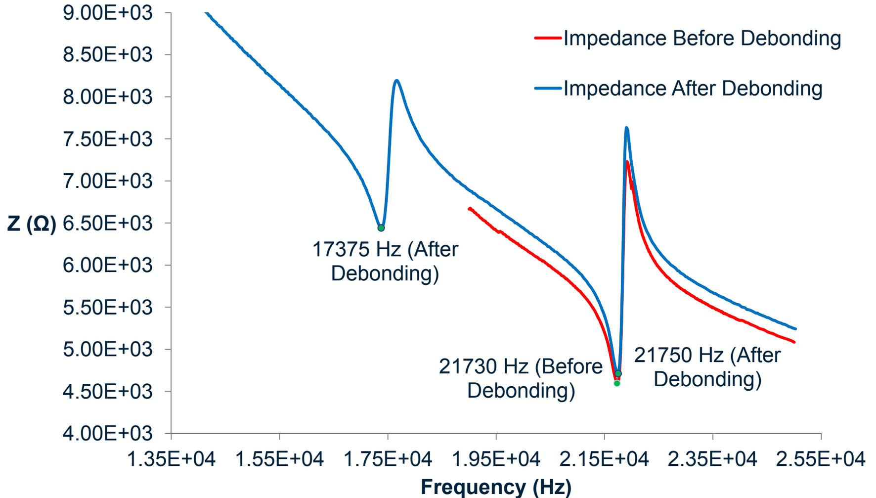
Impedance Analysis (Pre and Post Debonding) of the Standard Brass Cymbal Transducer
