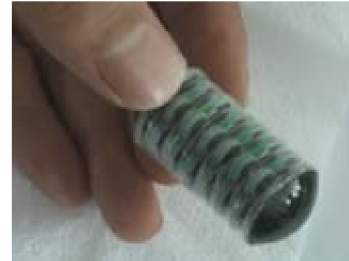
Smart pill that can crawl inside the gastronomical track
