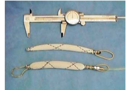
McKibben Artificial Muscles Air Pressure activation (B. Hannaford, Washington U.)
