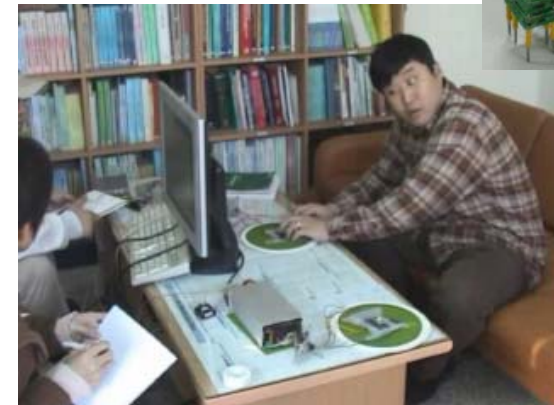
An EAP Braille display being tested by a blind person
