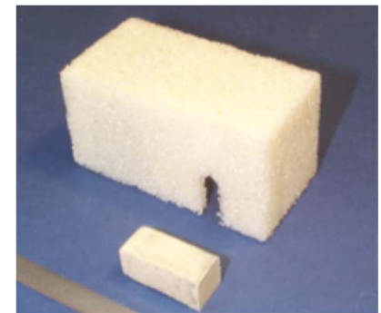
Shape Memory Polymers Heat/pressure activation (W. Sokolowski, JPL)
