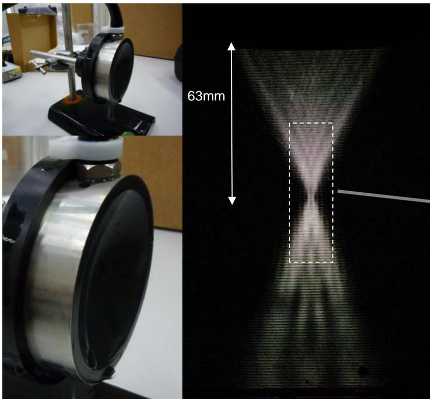
Pulse-pressure-squared integral around focus of Sonic Concepts 1.1 MHz transducer, using Onda Golden Lipstick 0.2mm hydrophone (transducer excited with 50 cycles, low drive levels to avoid hydrophone damage)
