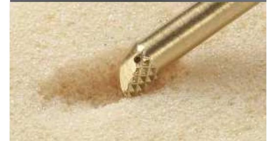
Relief exists, such that there is less resistance to cutting or cause of frictional drag and induced heating
