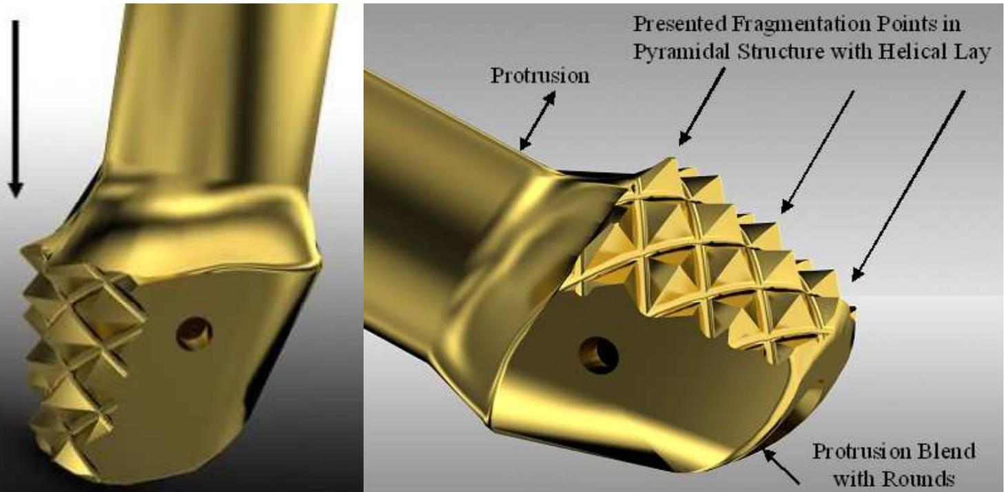
Relief exists, such that there is less resistance to cutting or cause of frictional drag and induced heating
