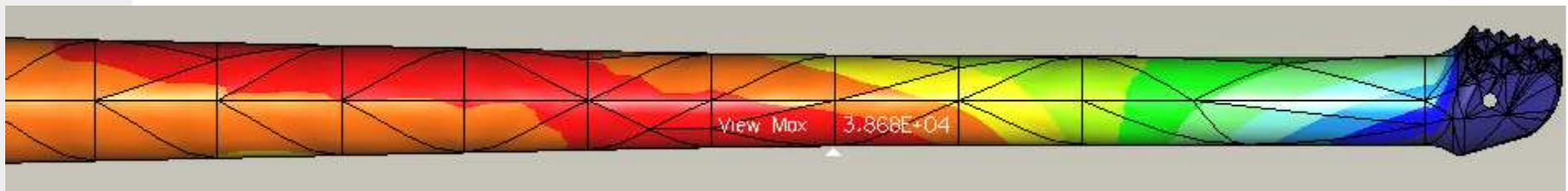
Maximum stress 268 MPa (38,700 Psi) due to longitudinal vibration and transverse ripple
