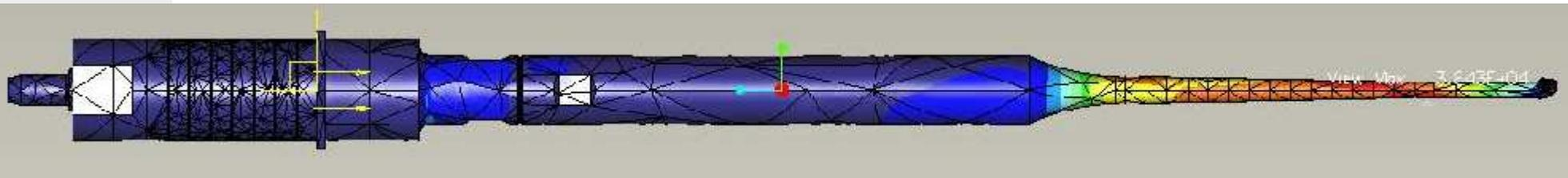
Transverse stress modulates longitudinal vibrational stress
