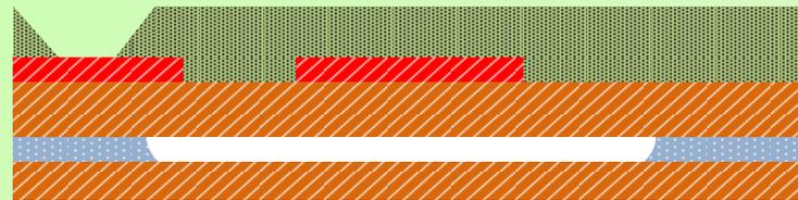
ZnO Sputtering deposition and open via access to bottom electrode through ZnO
