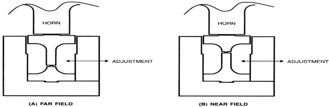
Figure 5—Energy Director Butt Joint Welding
