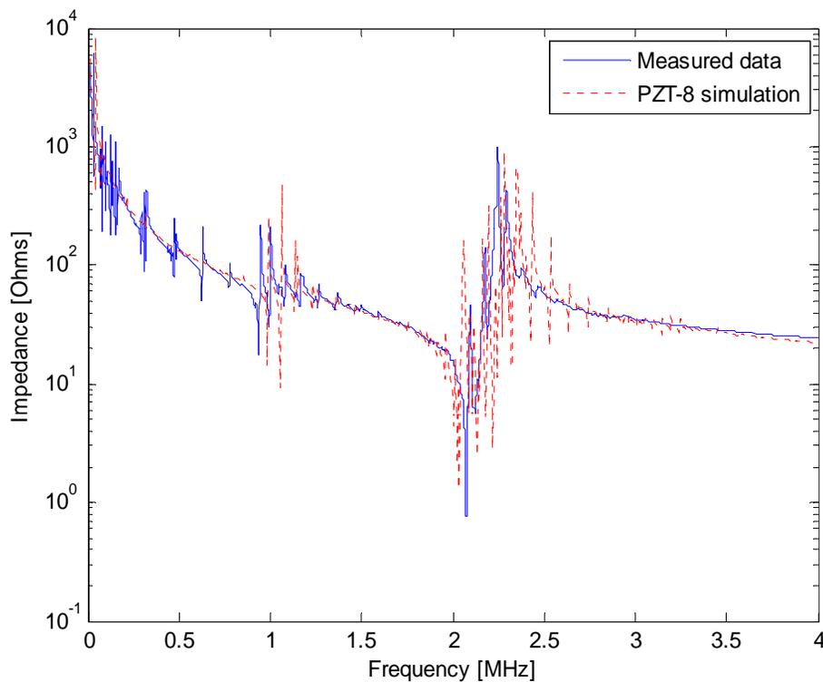
Electric impedance when transducer was emitting in air
