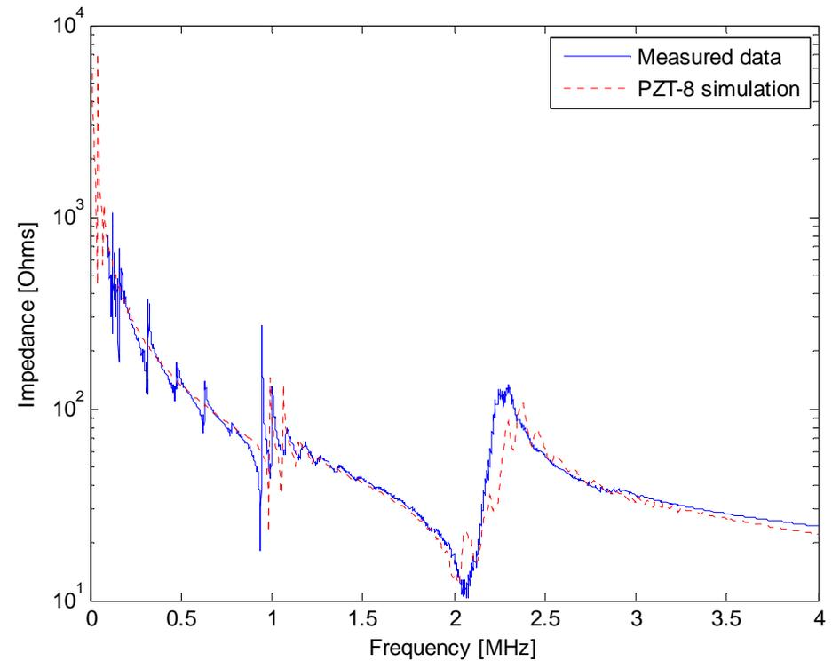
Electric impedance when transducer was emitting in water
