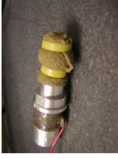
Wet chamois wrapped over horn Q = 25
