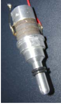
O rings slid over horn Q=150
