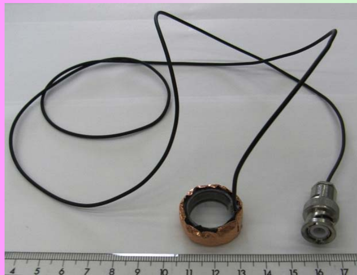
Fabricated cavitation sensor with hydrothermally synthesized PZT film
