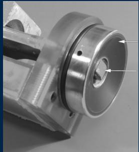
Sonic Concepts therapy 33 mm diameter 7.0 W to 9.3 W focal region 35 mm axial position 0.28 mm diameter 2.5 mm length
