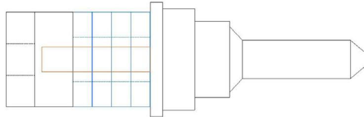
The 4 ring piezo stack (shown in blue) comprises the piezo elements and a beryllium copper shim electrode sandwiched between them. The complete stack including piezo, shim electrodes and joints, is treated as a single component. In the component editor, select Piezo Stack and note that the number of elements is the number of piezo rings that make up the stack.
