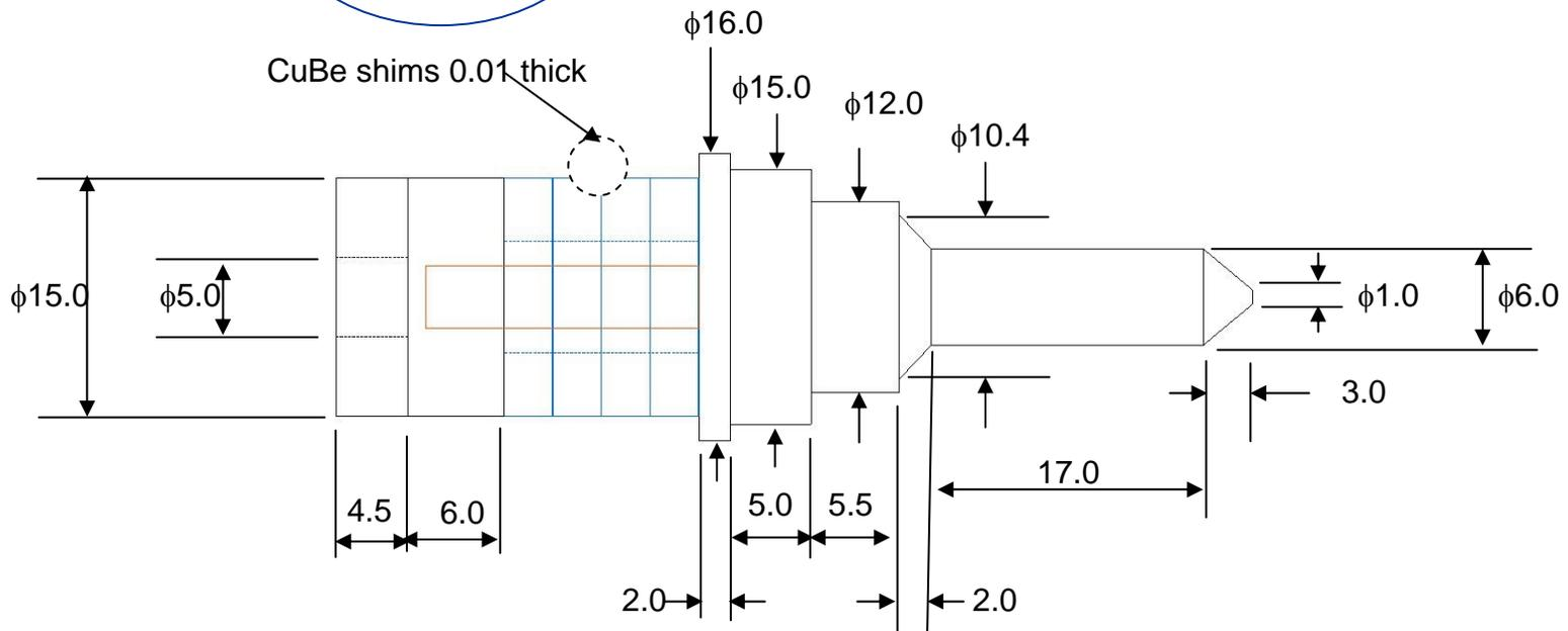
4 Navy Type I piezo rings  $\phi 15 \times \phi 7 \times 3$  (shown in blue)
