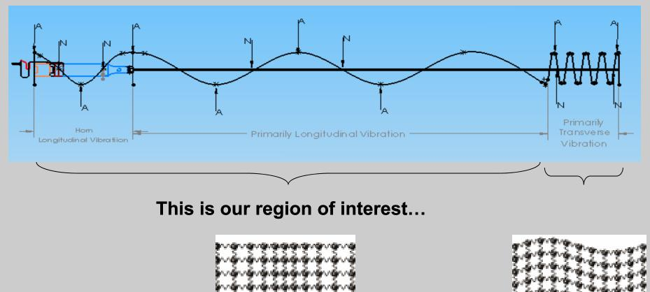
Converts longitudinal vibration generated by the transducer to transverse motion in the Wire's <u>Active Zone</u>
