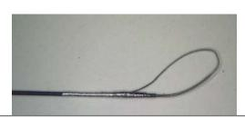
Nitinol Ribbon (0.0014- × 0.006in.) to Nitinol Tube (0.008-in. OD)
