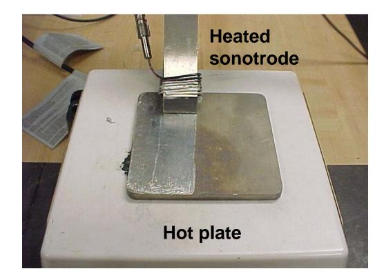
Ultrasonic pretinning oxidized Ti-6Al-4V
