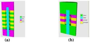
Figure 1: 2D Axisymmetric Transducer Models with PZT (a) and PMNPT (b)
