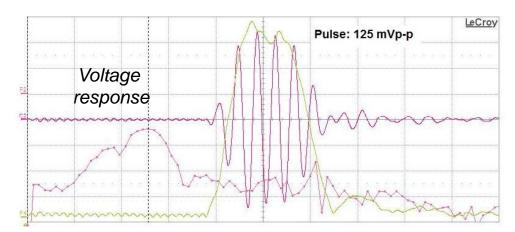
Pulse-echo response of single element from quartz flat. Centre Frequency: 51 MHz, Bandwidth: 25 %
