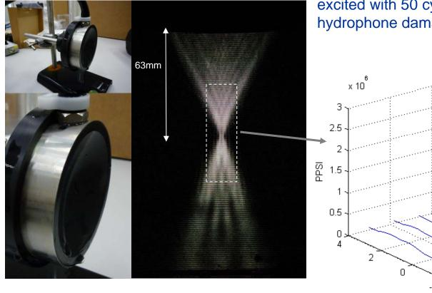
Pulse-pressure-squared integral around focus of Sonic Concepts 1.1 MHz transducer, using Onda Golden Lipstick 0.2mm hydrophone (transducer excited with 50 cycles, low drive levels to avoid hydrophone damage)
