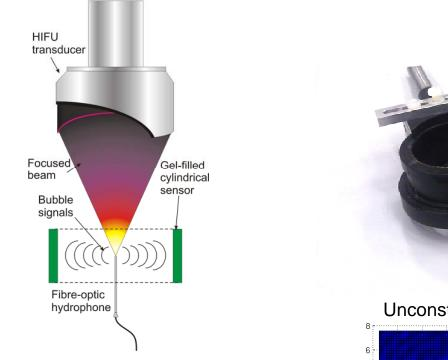
HIFU beam scanned across central plane and sensor response recorded
