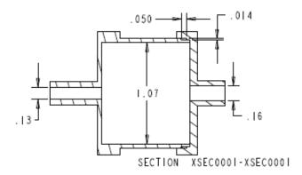
Common ultrasonic shear joint design.
