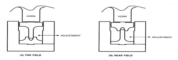
Figure 6—Double Shear Joint Welding
