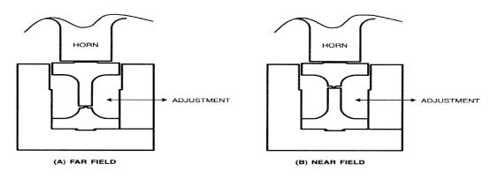
Figure 5—Energy Director Butt Joint Welding
