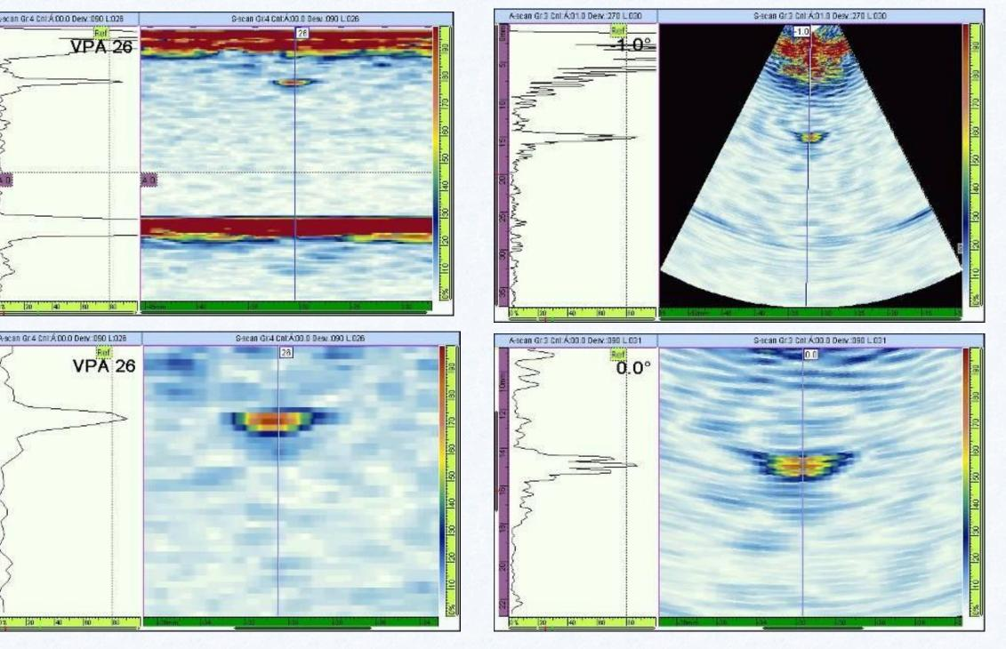
Fig. 2. Some array inspection results with Omniscan for an artificial flaw
