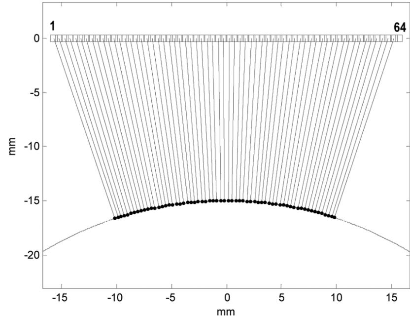
Detection of media boundary using ultrasound echo method
