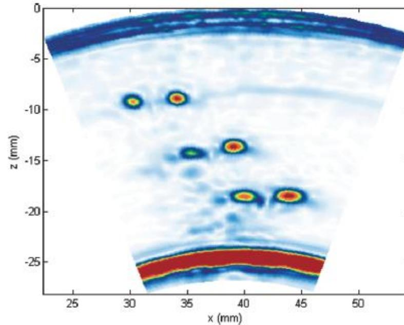
Aluminum ring with 3 pairs of SDH
