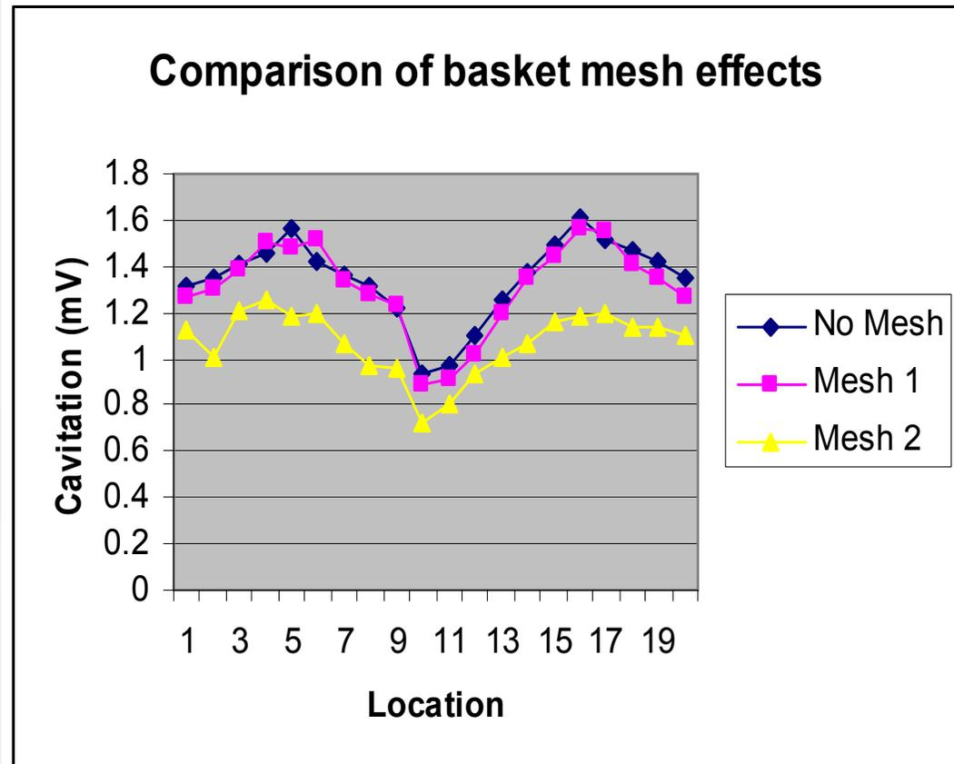
Figure (3): Effect of wire baskets on inertial cavitation.
