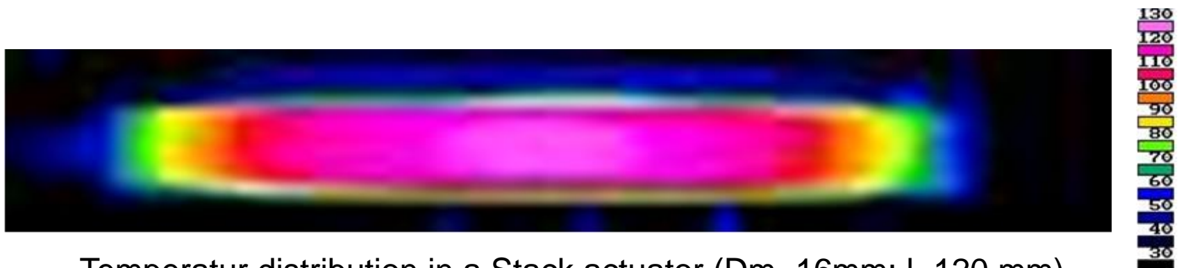
Temperatur distribution in a Stack actuator (Dm=16mm; l=120 mm)
