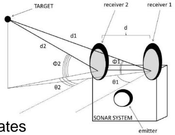
Target position in spherical coordinates
