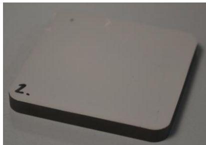
Ferroperm Hard PZ26 plate (Navy Type I), 50x50x5 mm (Meggit A/S)
