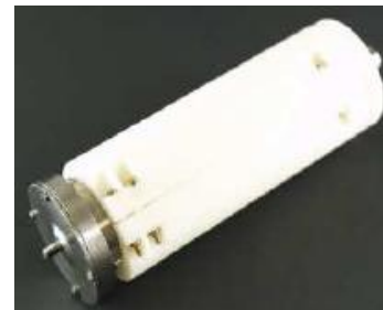
Surgical cutting application of a modified cymbal transducer (Bejarano et al., 2014)
