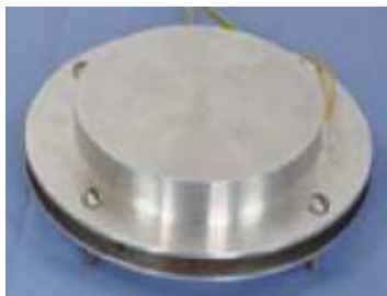
Flextensional modified for high amplitude (Lin, 2010)
