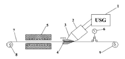
Fig. 1. A scheme of apparatus for wire drawing with superimposed ultrasonic vibrations: (1) ultrasonic generator, (2) ultrasonic transducer, (3) ultrasonic horn, (4) die, (5) pusher-type furnace, (6) dynamometer, (7) wire, (8, 9) spools.
