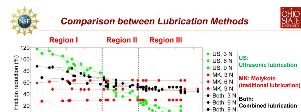
US lubrication depends on velocity but not load; MK depends on load but not ٠ velocity; Both combined are mostly invariant with changing velocity or load
