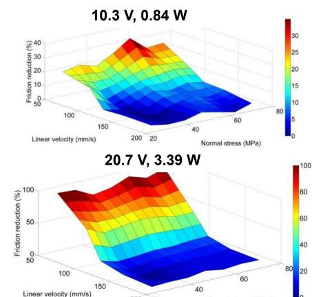
Friction reduction peaks at 48 and 55 MPa normal stress, especially at low velocities.
