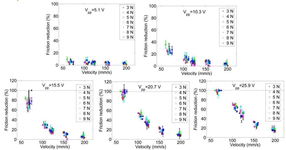
Note: Noise and measurement errors cause some data markers to show greater than 100% friction reduction.
