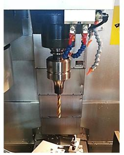
4.5kW module with shrink fit collet
