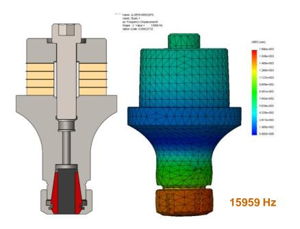
Note: Transducer/collet tuned low – brought to 20kHz with drill
