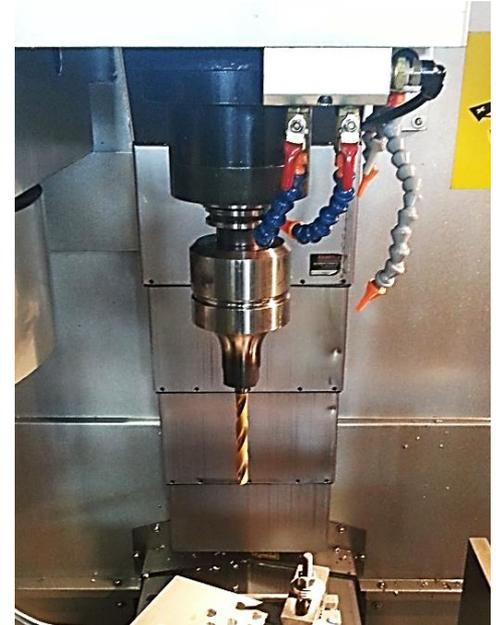
4.5kW module with shrink fit collet
