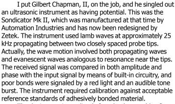
The device was immediately found to be capable of differentiating between well adhered adhesive in the lap joints and the lack of adhesive over moderate areas, including buttered over vacant regions. However further work was required to detect the present but nonadhered adhesive and also adhesive with weak bond(s).
